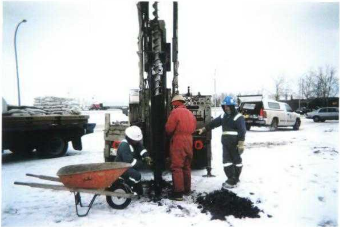
Photo No. 2 January 15 & 16, 2003; Phase III: Hydrocarbon ESA-Delineation Lots 5 &6, Block 28, Plan 3845 CO; 419 - 10 Avenue, Carstairs, Alberta Looking Southeast. Sampling Borehole #10.
