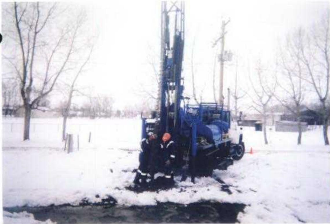
Photo No. 13: May 6, 2002; Phase II Hydrocarbon Environmental Site Assessment Lots 5 & 6, Block 28, Plan 3845 CO; 419 - 10 th Avenue, Carstairs, Alberta Looking West. Drilling Borehole #7/MW #3. Note: View of Urban Park West of the Subject Property, Across the Alley.
